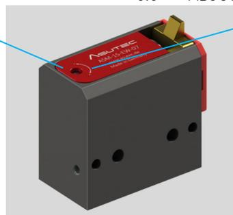
The damping effect can be adjusted on the top of the device at the ASM-15, ASM-20 and ASMHS-15 series by using a slotted screwdriver.
